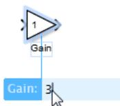
The hot parameter edit box allows you to enter a value for one parameter per block that you add using the quick insert feature.
